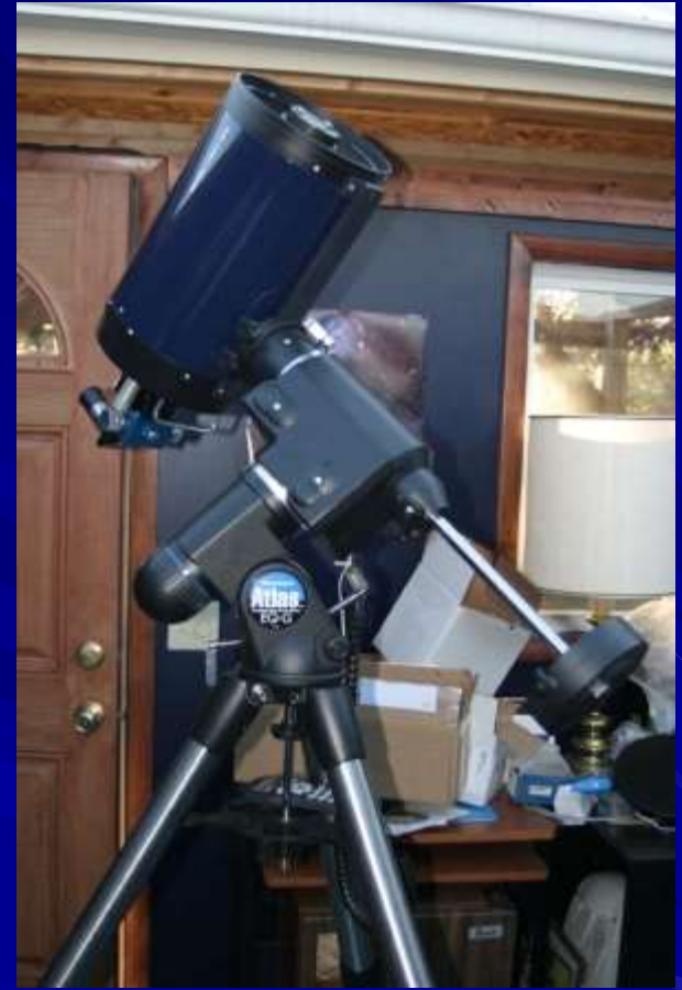
The 8" Ritchey-Chretien Cassegrain telescopes on Orion Atlas mounts are the workhorse of the department
